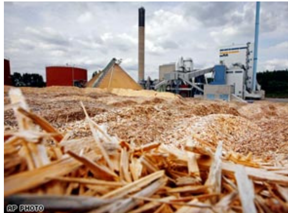
Fir and pine chips are piled high outside the electricity-and-heating plant in Vaxjo, Sweden.
