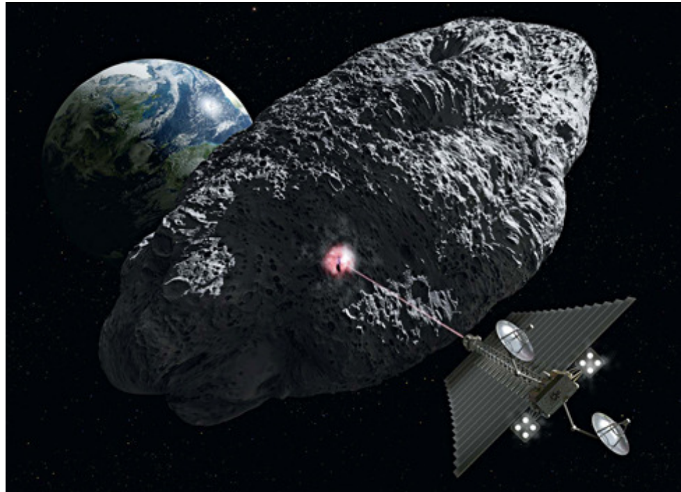
ROCK ROCKET A reflective solar mirror could concentrate solar energy on an asteroid, causing a patch to vaporize and act like a rocket thruster, knocking the rock off a collision course.
