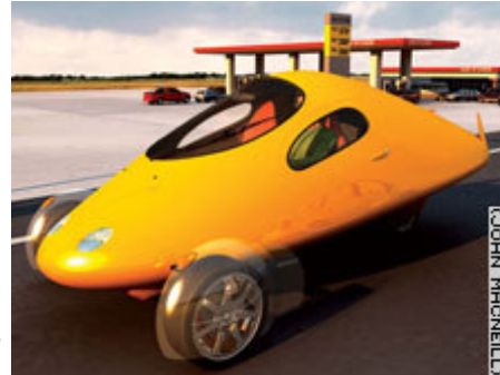
The Apera concept car uses a low-weight, low-drag approach to increasing fuel economy. The goal: 330 mpg for under $20,000 within two years.
