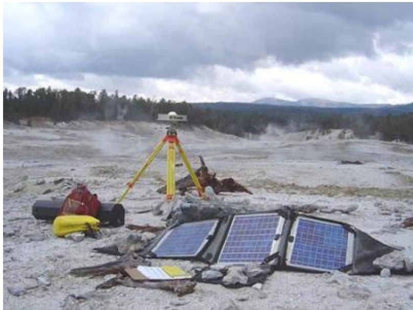
A Global Positioning System antenna measures gradual movements of the Earth's crust in Yellowstone National Park.
